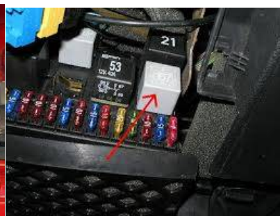
Fig.5 : Fuel Pump Relay
